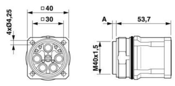
Pin version: dimension A = 3.8 mm, socket version: dimension A = 0.15 mm
