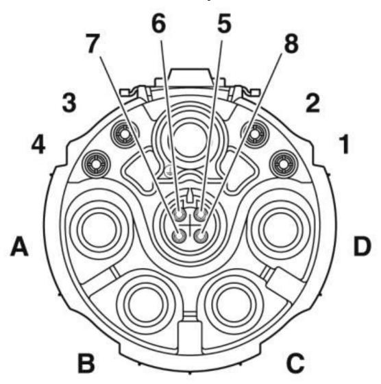
Pin assignment of socket signal, DC coding
