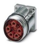
Device connector for front wall, SB, straight, shielded: yes, for standard and SPEEDCON interlock, M40, No. of pos.: 8+4+PE, type of contact: Socket, Crimp connection, Axial O-ring, 4x Ø4,2, flange dimensions: 40 mm x 40 mm
