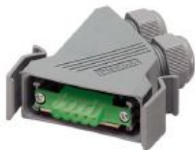
D-SUB complete connector, for DeviceNet, shell size 3, plug, screw connection, unshielded, connection direction straight, IP67 degree of protection
