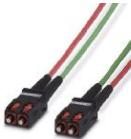
Assembled FO cable, breakout cable, 200/230 µm PCF fiber, SC-RJ/IP20 to SC-RJ/IP20, for installation inside control cabinets, length: 2 m
