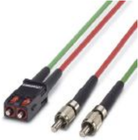
Assembled FO cable, breakout cable, 200/230 µm PCF fiber, SC-RJ/IP20 to FSMA/IP20, for installation inside control cabinets, length: 2 m
