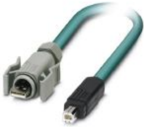
Assembled USB cable, shielded, color: RAL 5021 (water blue), PUR outer sheath, USB type A/IP67 on USB type B/standard, length: 5 m
