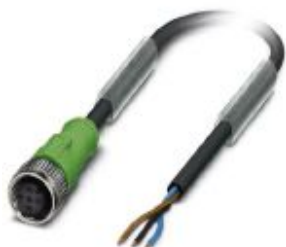
Sensor/actuator cable, 3-position, PUR halogen-free, black-gray RAL 7021, free cable end, on Socket straight M12, coding: A, PIN 2+4 bridged, cable length: 3 m
