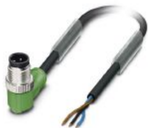
Sensor/actuator cable, 3-position, PUR halogen-free, black-gray RAL 7021, Plug angled M12, coding: A, on free cable end, cable length: 1.5 m
