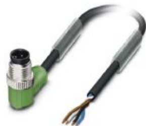
Sensor/actuator cable, 4-position, PUR halogen-free, black-gray RAL 7021, Plug angled M12, coding: A, on free cable end, cable length: 1.5 m
