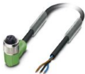
Sensor/actuator cable, 3-position, PUR halogen-free, black-gray RAL 7021, free cable end, on Socket angled M12, coding: A, PIN 2+4 bridged, cable length: 3 m
