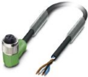
Sensor/actuator cable, 4-position, PUR halogen-free, black-gray RAL 7021, free cable end, on Socket angled M12, coding: A, cable length: 1.5 m
