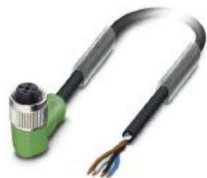
Sensor/actuator cable, 4-position, PUR halogen-free, black-gray RAL 7021, free cable end, on Socket angled M12, coding: A, cable length: 3 m
