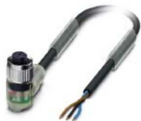
Sensor/actuator cable, 3-position, PUR halogen-free, black-gray RAL 7021, free cable end, on Socket angled M12, coding: A, with 2 LEDs, PIN 2+4 bridged, cable length: 5 m
