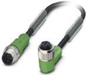
Sensor/actuator cable, 3-position, PUR halogen-free, black-gray RAL 7021, Plug straight M12, coding: A, on Socket angled M12, coding: A, PIN 2+4 bridged, cable length: 0.3 m
