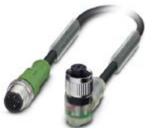
Sensor/actuator cable, 3-position, PUR halogen-free, black-gray RAL 7021, Plug straight M12, coding: A, on Socket angled M12, coding: A, with 2 LEDs, PIN 2+4 bridged, cable length: 0.6 m
