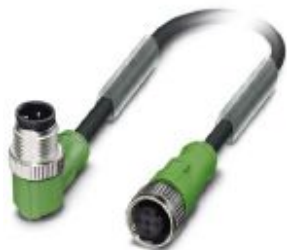
Sensor/actuator cable, 3-position, PUR halogen-free, black-gray RAL 7021, Plug angled M12, coding: A, on Socket straight M12, coding: A, PIN 2+4 bridged, cable length: 0.6 m
