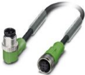
Sensor/actuator cable, 4-position, PUR halogen-free, black-gray RAL 7021, Plug angled M12, coding: A, on Socket straight M12, coding: A, cable length: 3 m
