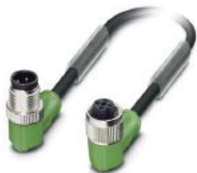
Sensor/actuator cable, 3-position, PUR halogen-free, black-gray RAL 7021, Plug angled M12, coding: A, on Socket angled M12, coding: A, PIN 2+4 bridged, cable length: 0.3 m
