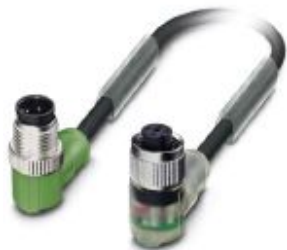
Sensor/actuator cable, 4-position, PUR halogen-free, black-gray RAL 7021, Plug angled M12, coding: A, on Socket angled M12, coding: A, with 3 LEDs, cable length: 1.5 m
