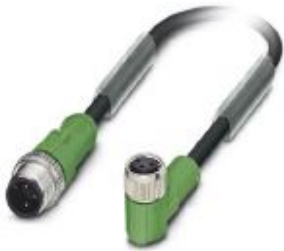
Sensor/actuator cable, 3-position, PUR halogen-free, black-gray RAL 7021, Plug straight M12, coding: A, on Socket angled M8, cable length: 3 m
