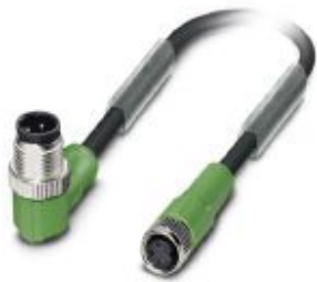
Sensor/actuator cable, 3-position, PUR halogen-free, black-gray RAL 7021, Plug angled M12, coding: A, on Socket straight M8, cable length: 1.5 m
