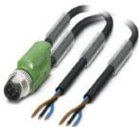
Sensor/actuator cable, 3-position, PUR halogen-free, black-gray RAL 7021, unshielded, Plug straight M12, coding: A, on free cable end and free cable end, cable length: 1.5 m
