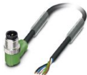
Sensor/actuator cable, 5-position, PUR halogen-free, black-gray RAL 7021, Plug angled M12, coding: A, on free cable end, cable length: 1.5 m
