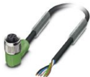
Sensor/actuator cable, 5-position, PUR halogen-free, black-gray RAL 7021, free cable end, on Socket angled M12, coding: A, cable length: 1.5 m
