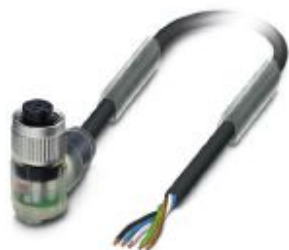
Sensor/actuator cable, 5-position, PUR halogen-free, black-gray RAL 7021, free cable end, on Socket angled M12, coding: A, with 3 LEDs, cable length: 1.5 m
