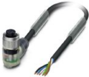
Sensor/actuator cable, 5-position, PUR halogen-free, black-gray RAL 7021, free cable end, on Socket angled M12, coding: A, with 3 LEDs, cable length: 3 m
