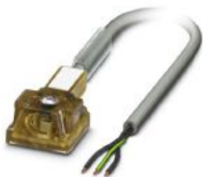
Sensor/actuator cable, 3-position, PUR/PVC, gray RAL 7001, free cable end, on Valve connector A, with 1 LED, connected with Z diode, cable length: 3 m
