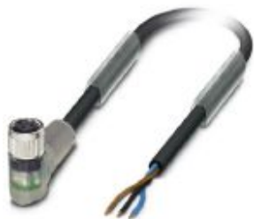
Sensor/actuator cable, 3-position, PUR halogen-free, black-gray RAL 7021, free cable end, on Socket angled M8, with 2 LEDs, cable length: 3 m
