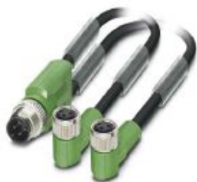
Sensor/actuator cable, 3-position, PUR halogen-free, black-gray RAL 7021, Plug straight M12, coding: A, on Socket angled M8 and Socket angled M8, coding: A, cable length: 0.3 m
