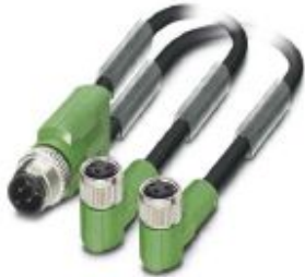
Sensor/actuator cable, 3-position, PUR halogen-free, black-gray RAL 7021, Plug straight M12, coding: A, on Socket angled M8 and Socket angled M8, coding: A, cable length: 0.6 m
