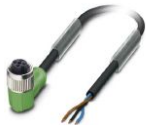
Sensor/actuator cable, 3-position, PUR halogen-free, black-gray RAL 7021, free cable end, on Socket angled M12, coding: A, PIN 2+4 bridged, cable length: 10 m
