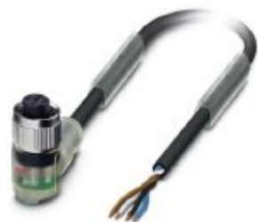
Sensor/actuator cable, 4-position, PUR halogen-free, black-gray RAL 7021, free cable end, on Socket angled M12, coding: A, with 3 LEDs, cable length: 10 m
