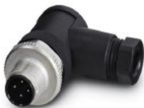
Connector, Universal, Universal, 4-position, Plug angled M12, Coding: A, Screw connection, knurl material: Zinc die-cast, nickel-plated, cable gland Pg7, external cable diameter 4 mm ... 6 mm
