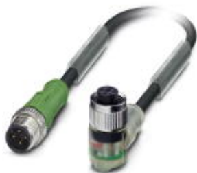
Sensor/actuator cable, 4-position, PUR halogen-free, black-gray RAL 7021, Plug straight M12, A-coded, on Socket angled M12, A-coded, with 3 LEDs, cable length: 5 m
