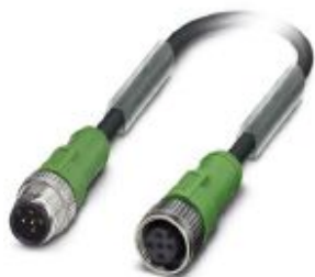
Sensor/actuator cable, 5-position, PUR halogen-free, black-gray RAL 7021, Plug straight M12, coding: A, on Socket straight M12, coding: A, cable length: 0.6 m
