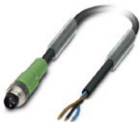
Sensor/actuator cable, 3-position, PUR halogen-free, black-gray RAL 7021, Plug straight M8, on free cable end, cable length: 1.5 m
