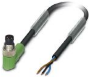
Sensor/actuator cable, 3-position, PUR halogen-free, black-gray RAL 7021, Plug angled M8, on free cable end, cable length: 1.5 m
