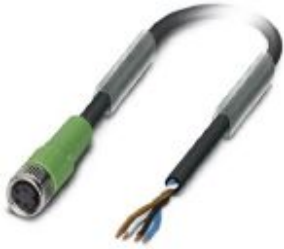
Sensor/actuator cable, 4-position, PUR halogen-free, black-gray RAL 7021, free cable end, on Socket straight M8, cable length: 1.5 m
