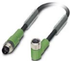
Sensor/actuator cable, 3-position, PUR halogen-free, black-gray RAL 7021, Plug straight M8, on Socket angled M8, cable length: 1.5 m
