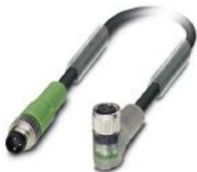
Sensor/actuator cable, 3-position, PUR halogen-free, black-gray RAL 7021, Plug straight M8, on Socket angled M8, with 2 LEDs, cable length: 1.5 m
