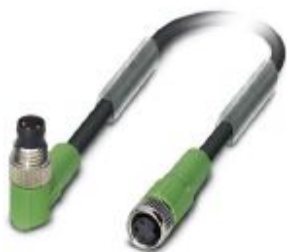
Sensor/actuator cable, 3-position, PUR halogen-free, black-gray RAL 7021, Plug angled M8, on Socket straight M8, cable length: 0.3 m
