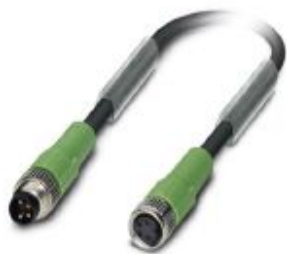
Sensor/actuator cable, 4-position, PUR halogen-free, black-gray RAL 7021, Plug straight M8, on Socket straight M8, cable length: 0.3 m
