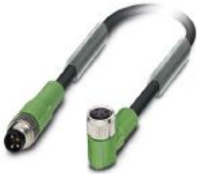
Sensor/actuator cable, 4-position, PUR halogen-free, black-gray RAL 7021, Plug straight M8, on Socket angled M8, cable length: 3 m
