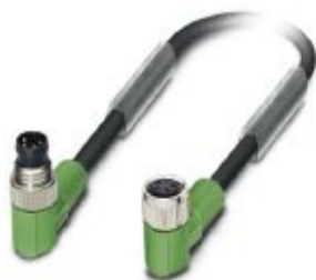
Sensor/actuator cable, 4-position, PUR halogen-free, black-gray RAL 7021, Plug angled M8, on Socket angled M8, cable length: 1.5 m
