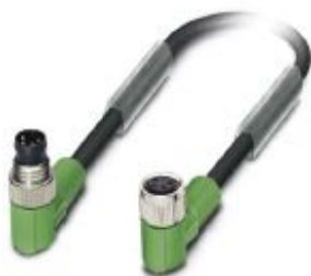
Sensor/actuator cable, 4-position, PUR halogen-free, black-gray RAL 7021, Plug angled M8, on Socket angled M8, cable length: 3 m
