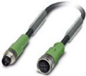
Sensor/actuator cable, 3-position, PUR halogen-free, black-gray RAL 7021, Plug straight M8, on Socket straight M12, coding: A, cable length: 0.3 m
