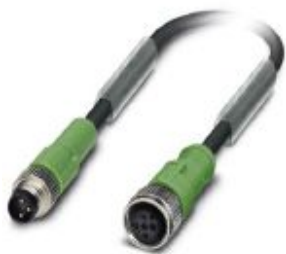
Sensor/actuator cable, 3-position, PUR halogen-free, black-gray RAL 7021, Plug straight M8, on Socket straight M12, coding: A, cable length: 3 m
