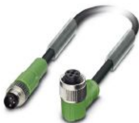
Sensor/actuator cable, 3-position, PUR halogen-free, black-gray RAL 7021, Plug straight M8, on Socket angled M12, coding: A, cable length: 0.6 m
