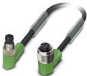
Sensor/actuator cable, 3-position, PUR halogen-free, black-gray RAL 7021, Plug angled M8, on Socket angled M12, coding: A, cable length: 0.6 m
