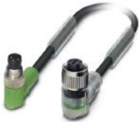
Sensor/actuator cable, 3-position, PUR halogen-free, black-gray RAL 7021, Plug angled M8, on Socket angled M12, coding: A, with 2 LEDs, cable length: 1.5 m
