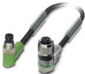
Sensor/actuator cable, 3-position, PUR halogen-free, black-gray RAL 7021, Plug angled M8, on Socket angled M12, coding: A, with 2 LEDs, cable length: 3 m
